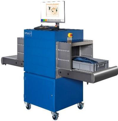
HI-SCAN 5030C is a compact, lightweight X-ray inspection system designed for easy transportability. It is available in a mobile or table-top configuration. The tunnel size of 532mm (W) x 328mm (H) accommodates mail including envelopes and small packages. This system is ideal for detecting weapons, explosives, and other visible threats.
