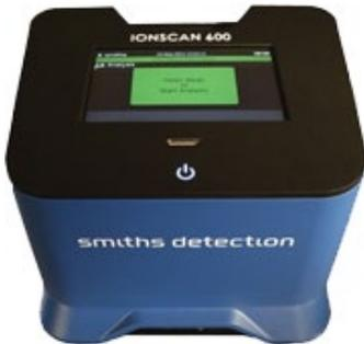
IONSCAN 600 is a portable ion-mobility spectrometry system designed to detect trace amounts of threat substances not visible to the naked eye. The system can be configured for narcotics, explosives or dual mode libraries of contraband substances. IONSCAN 600 can be used to screen envelopes and parcels of all sizes and delivers analysis results in 8 seconds.
