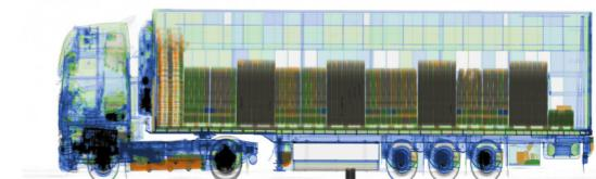
Differentiate organic and inorganic materials through colour. By using advanced colourisation, the system highlights materials concealed within cargo, providing operators with clear, actionable visual information for faster and more accurate analysis.
