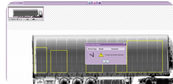
A suite of advanced software enhancements that provides image operators with automatic and assisted recognition of targets and potential threats. Current automatic detection capabilities include cigarette identification, non-homogeneous cargo recognition and empty or partially filled container detection.
