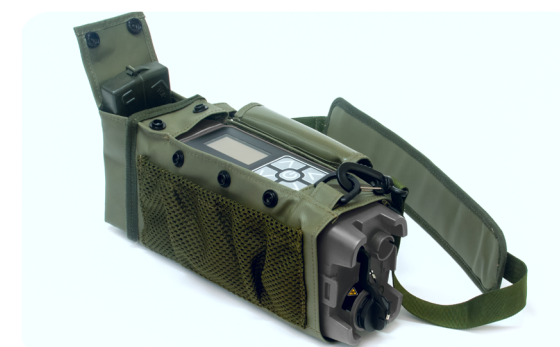
Trace solid and liquid threat detection (LCD 4 XID adapter)
