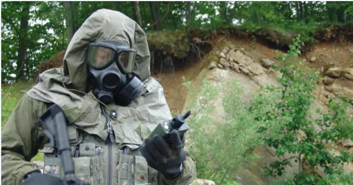
LCD 4 takes less than 90 seconds to become mission available, will run for up to 96 hours on commercial AA batteries and holds at least 72 hours of detection data. The LCD 4 can be rapidly shut down at any time without detriment to the equipment.
