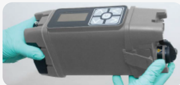
Clip front cover in place and power on the LCD 4 XID.
