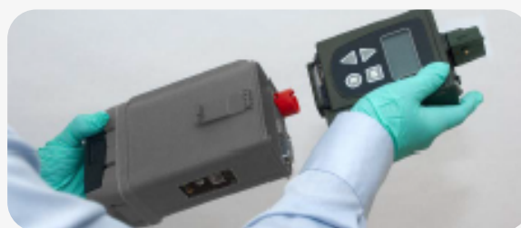
Slide LCD 4 into XID adapter.
