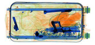
Automatic detection of gun parts using iCMORE Weapons on a HI-SCAN 6040aTiX
