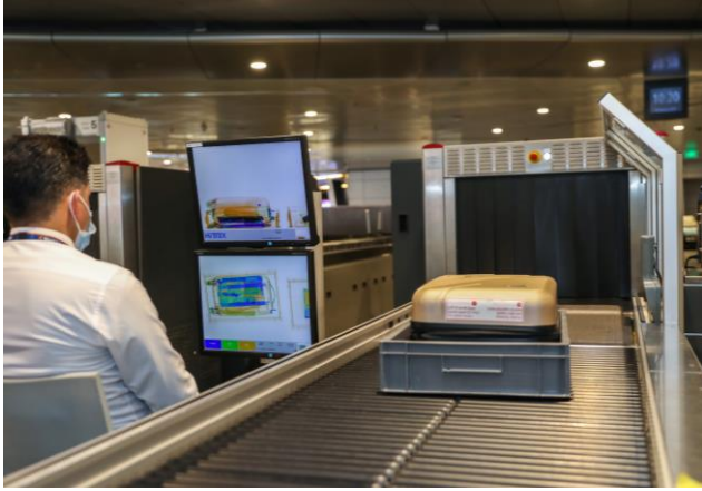
The HI-SCAN 7555aTiX provides two detailed high-resolution views, and an automatic detection of solid and liquid explosives during the screening of carry-on baggage.
