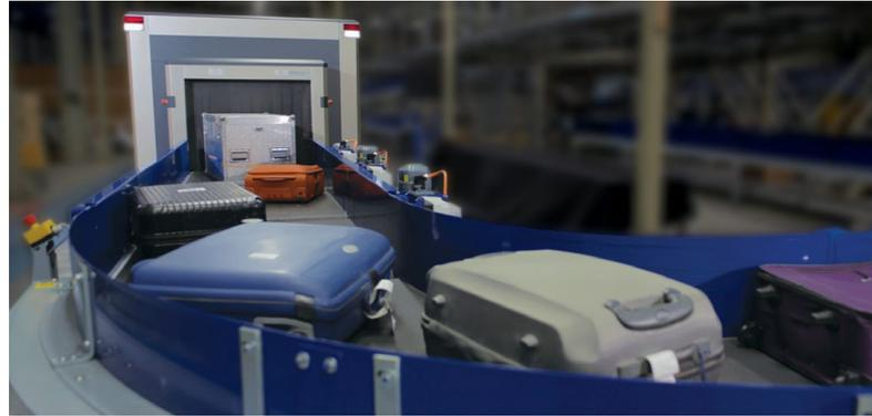
The HI-SCAN 10080 XCT CT HBS scanner can screen up to 1,800 bags per hour.
