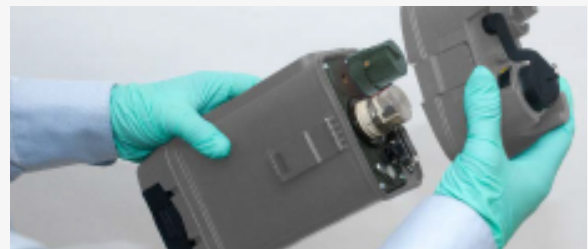
Position XID front cover over top of LCD 4.
