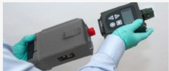
Slide LCD 4 into XID adapter.
