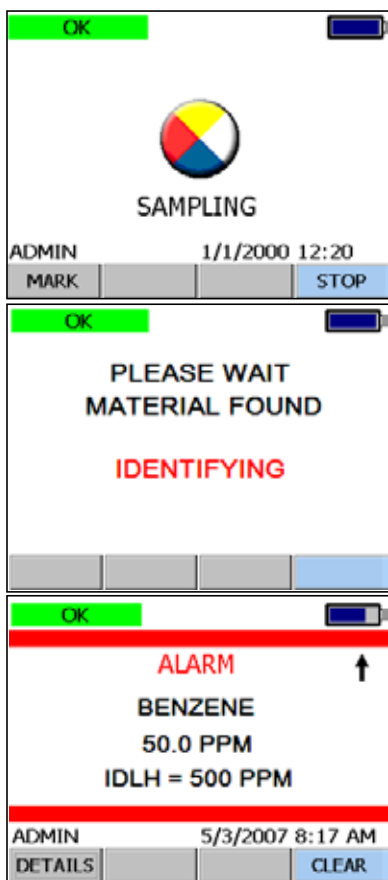
Figure 3. Screen Shot Sequence of Chemical Identification: Sampling, Detection and Identification
