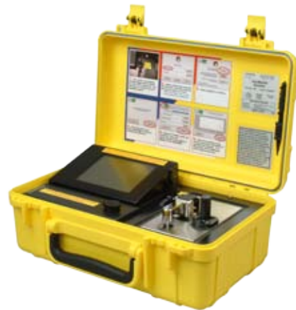
Figure 2 The HazMatID™, a rugged and portable FT-IR chemical identifier
